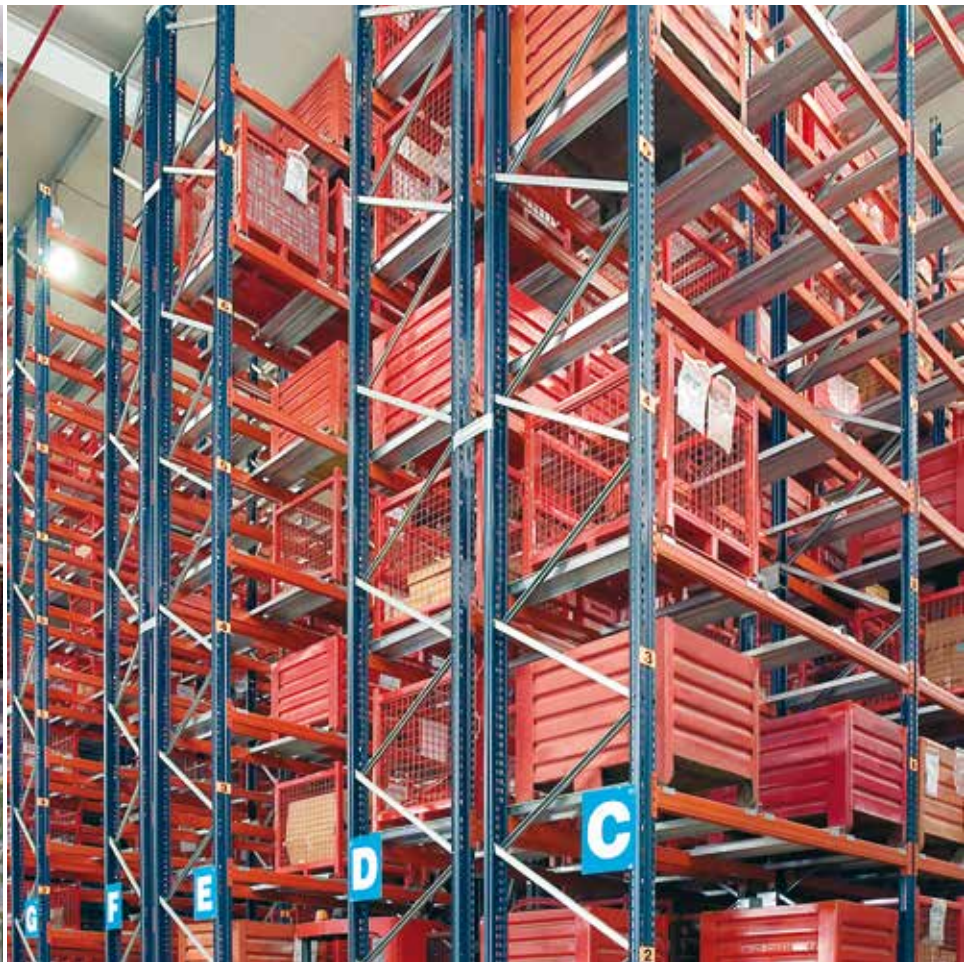
Selective pallet racking system with metal containers
