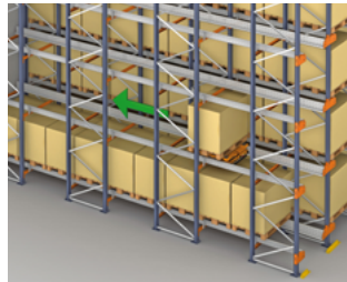
STEP 3 The shuttle raises one pallet slightly and then moves horizontally until reaching the first open location, where it sets the pallet down.
