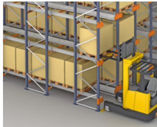
STEP 2 The forklift loads the pallets one by one at the level's entrance, supporting them on the loading sections.
